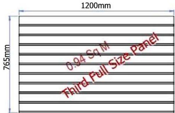
1200 x 765mm Tracker Panels for 65mm brick Slips 3mm Deep with 10mm Mortar Joints
