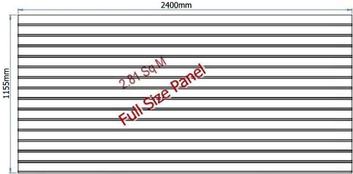
2400 x 1155mm Tracker Panels for 65mm brick Slips 3mm Deep with 10mm Mortar Joints
