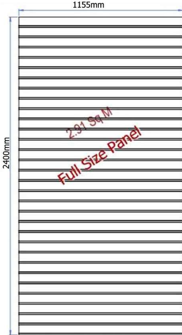
2400 x 1155mm Tracker Panels for 65mm brick Slips 3mm Deep with 10mm Mortar Joints
