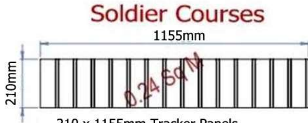
210 x 1155mm Tracker Panels for 65mm brick Slips 3mm Deep with 10mm Mortar Joints
