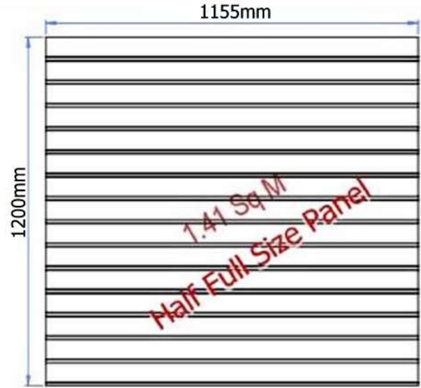
1200 x 1155 Tracker Panels for 65mm brick Slips 3mm Deep with 10mm Mortar Joints
